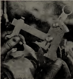
Gage Used on Diameter of 4-Inch Helical Mill
